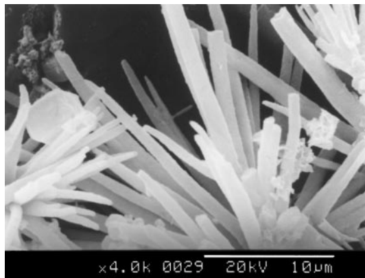
Fig. 1 Scanning electron microscopy (Hitachi, model S-2300) image of SiO 2 -CNT glass rods.
